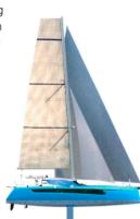
Builder: Slyder Catamarans - Length: 59' (17.99 m) - Beam: 28'6" (8.68 m) - Draft: 4'3"/8'10" (1.3/2.7 m) - Light displacement: 39,250 lbs (17.8 t) - Mainsail: 1.130 sq ft (105 m<sup>2</sup>) - Genoa: 721 sq ft (67 m<sup>2</sup>) Gennaker: 2,205 sq ft (205 m<sup>2</sup>) - Motors: 2 x 25 kW - Price: tba
