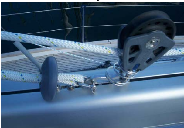
Incorrect position – will scratch the boom
