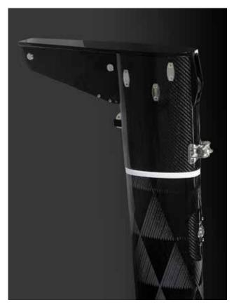
stretch sails with a good service life. The main has an impressive headboard and generous roach, creating a powerful sail with proportions that are only possible with a big carbon crane on the back of the mast head, to allow enough space between the leach and the backstay. This takes the performance of in-mast furling another step forward.
