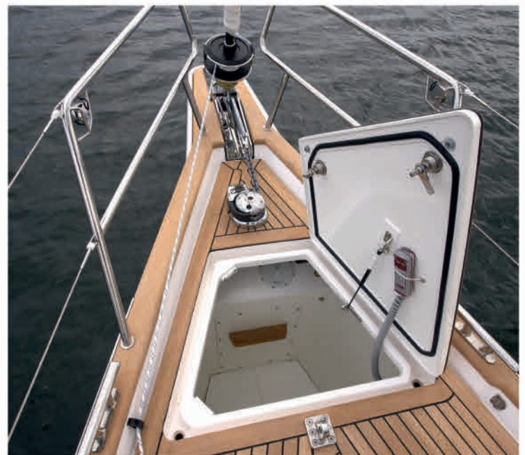
In the foredeck a deep sail locker, with integrated self-draining anchor chain compartment. The electrical anchor winch capstan can be fitted with an optional topwinch to operate moorings.
