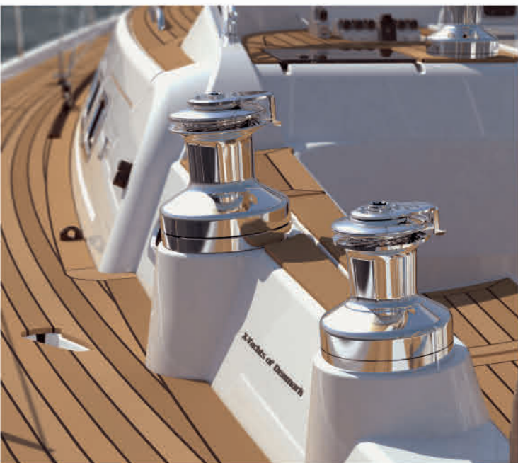
Stainless steel self-tailing Andersen Winches, which can be upgraded to be electrical powered, are part of Xc 45's comprehensive standard quality.
